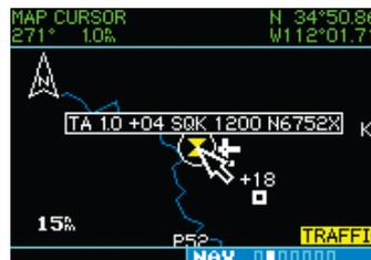
When the target pointer is placed on traffic, the traffic range, squawk code (if available), and tail number (if available) are displayed.
