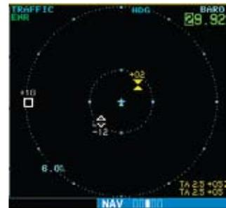
The Barometric Pressure field is located in the upper right-hand corner of the Traffic Page.
