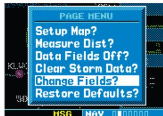
The Map Page can display TCAD traffic in any of the top three fields (or top four fields on a 500W Series unit) located on the right-hand side of the display.
