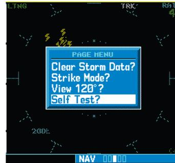
In addition to the power-up test, the user can perform a self-test that is executed through the 400W/500W Series unit display.
