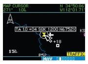
When the target pointer is placed on traffic, the traffic range, squawk code (if available), and tail number (if available) are displayed.
