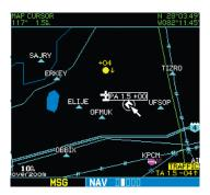
When the target pointer is placed on traffic, the traffic range and altitude separation are displayed.
