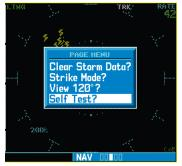
In addition to the power-up test, the user can perform a self-test that is executed through the 400W/500W Series unit display.
