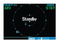
The Standby Screen appears when the SKYWATCH passes the power-up test. NOTE: when the system is in standby, the SKY-WATCH does not transmit, interrogate, or track intruders aircraft.
